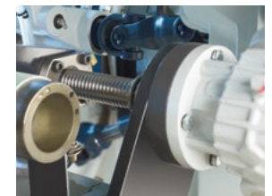
Positioning axes with ball screw and encoder
